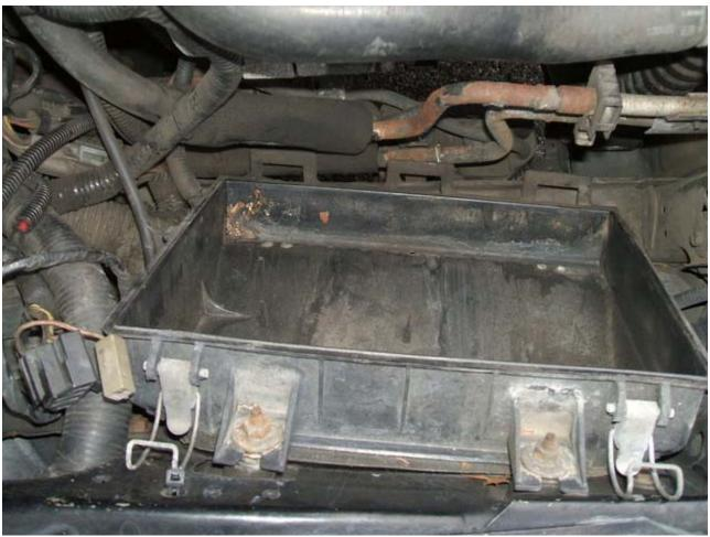
Install the new filter in the filter housing. I like to mark the date and mileage on the filter.
