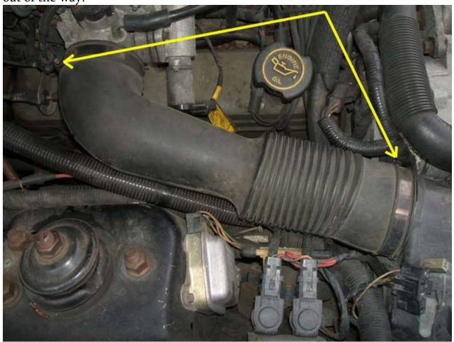
Unfasten the four clips (two on the top and one on each side) to remove the air cleaner lid.
