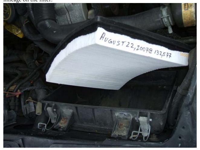
Ensure that the filter is completely seated into the housing.
