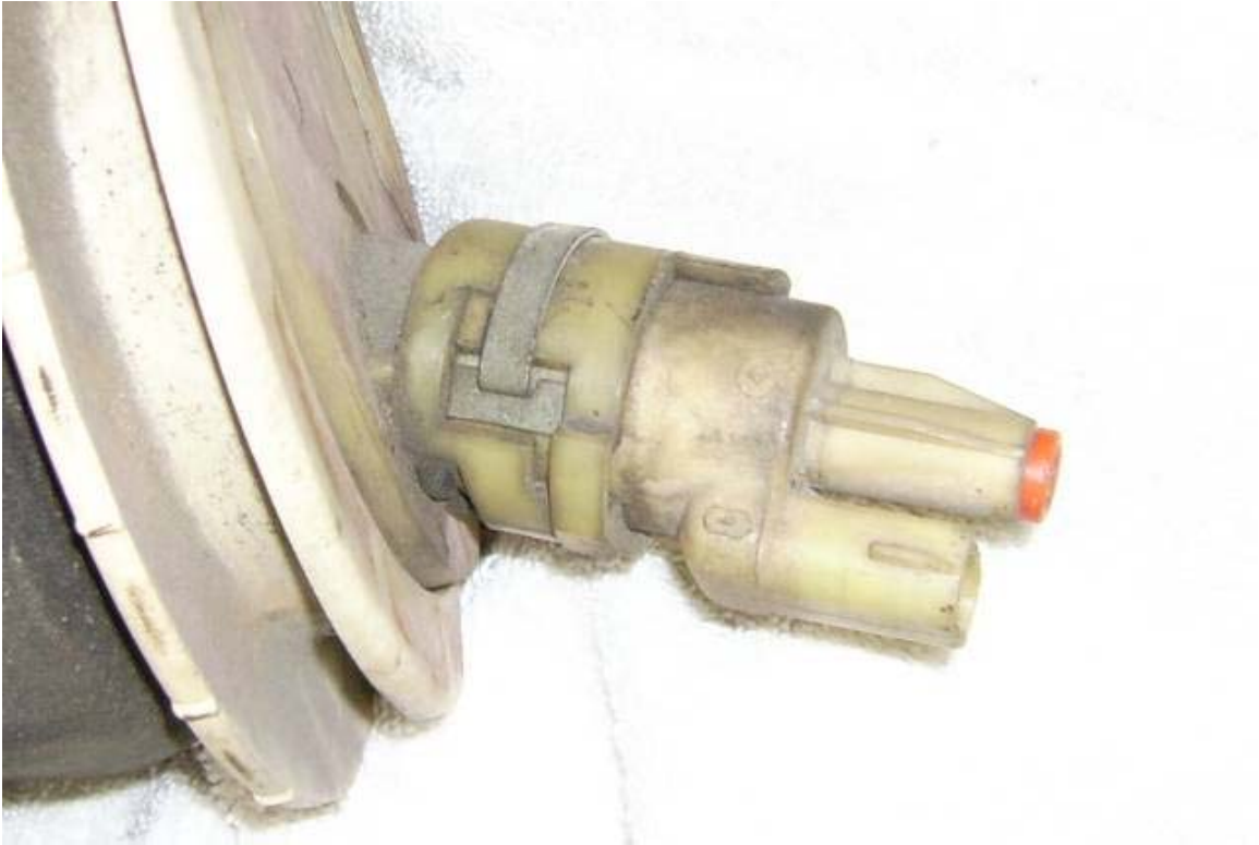
Solenoid Installed in Air Spring (Typical)
