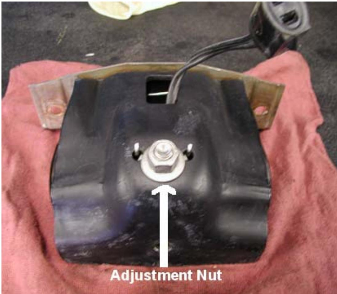
The large nut in the center is the adjustment nut. By loosening this nut, you can aim the fog light. Grab a 15mm socket or wrench and remove this nut. The tension springs are behind the light and the light must be removed to get to them.
