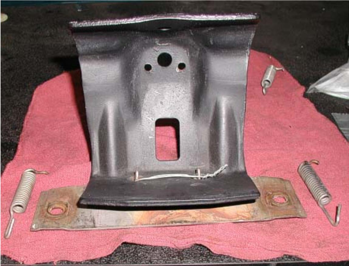
Put the bracket assembly in a vise and secure it. The new springs will be MUCH tighter than the old springs. Insert the long end in the pivot mount, hold the short end with a pair of needle nose pliers and stretch so the small end fits thru the retaining hole. A small punch may help push the spring through the hole.
