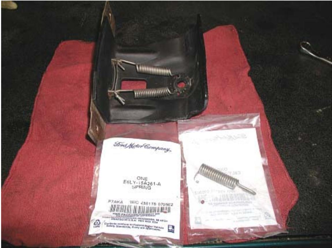
With a pair of needle nose pliers, grab the short end of the spring and pull out of the retaining hole. Pay attention to the position in which they were, the new springs must go back in the same position. Both springs can be removed at the same time and the bracket disassembled for detailing.
